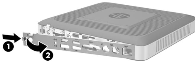
8. Move the access panel latch (1) to the right to release the access panel.
