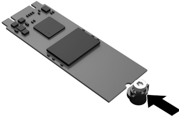
12. Slide the new storage module into the M.2 socket on the system board and press the module connectors firmly into the socket.
